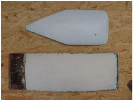
Sailing Blade mould after some use and ready to go. The auxiliary mould at the top has been taken from a moulded blade.
