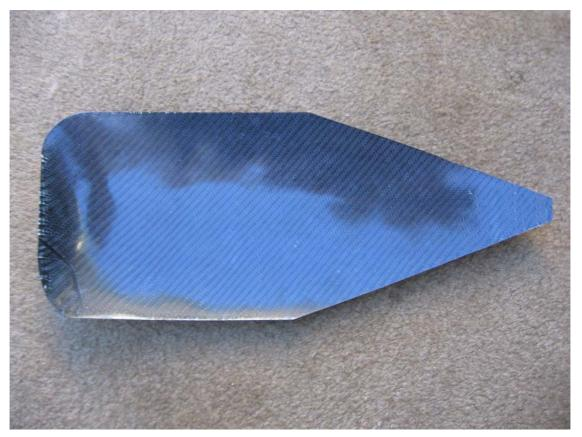
The finished job trimmed with an angle grinder cutting wheel, weighs only 200 grams (7oz.) and is pretty well unbreakable.
