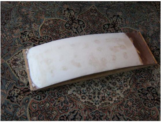
The Sailing blade mould before fibre glassing.
