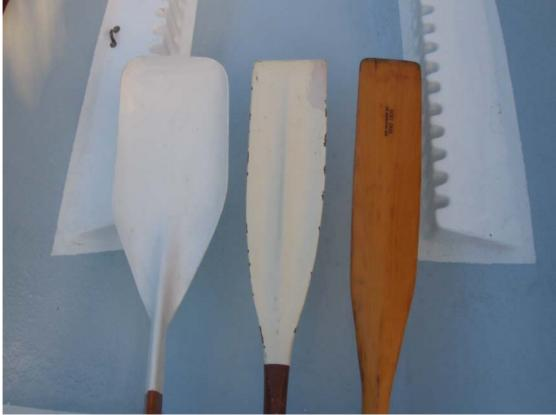
Oars from right to left are, Flat blade, Spoon blade and carbon fibre Turbo blade.
