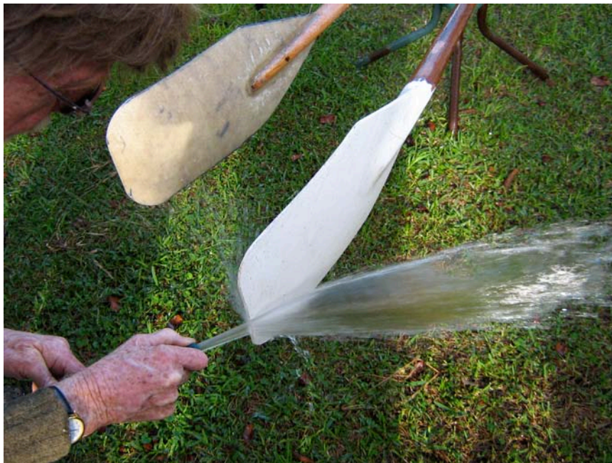
The water does not attach to the rear of a more conventional blade.
