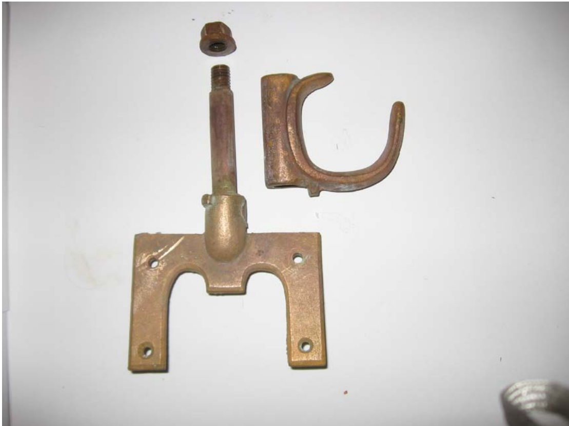
A more rugged design of oarlock.
