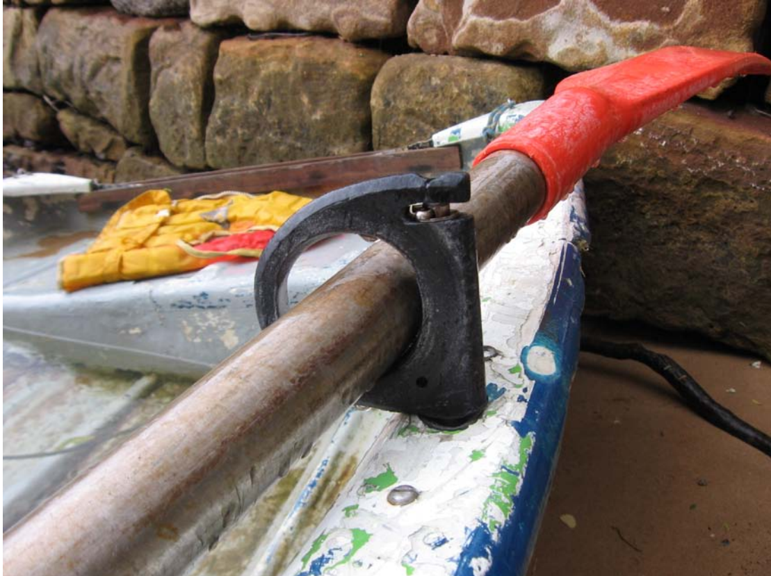
Hand made oarlock after 20 years of use. (The plastic rotates around the pin so the pin does not move in the socket.)
