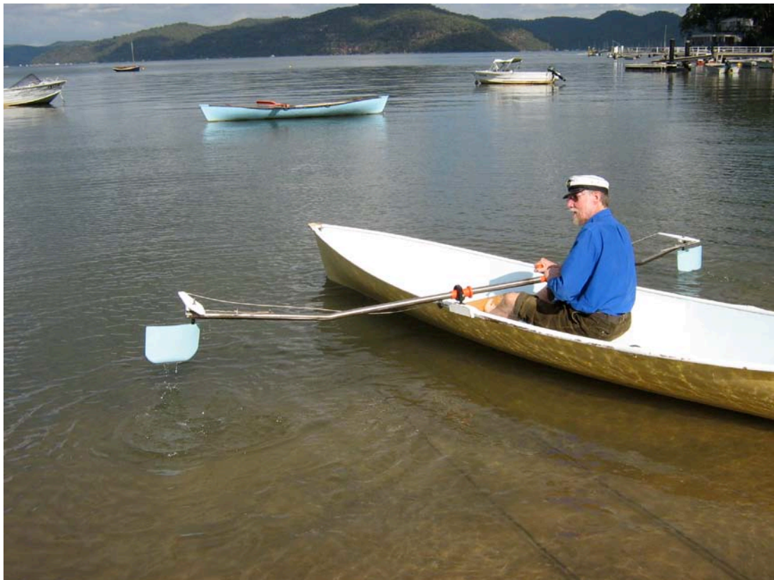
The blade swivels at right angles to travel. Its angle is controlled by a lanyard attached to the gunwale.
