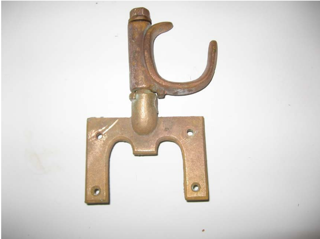
Assembled oarlock is squeaky without grease.
