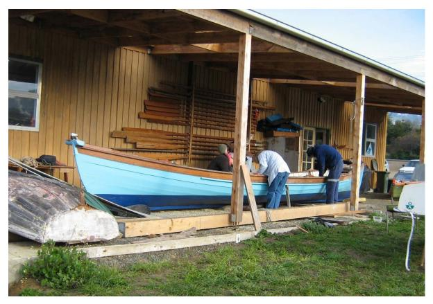
Thirty four foot replica of a six oar, NZ bay whaler, built by The Living Boat Trust, Franklin, Tasmania. Note the different oar lengths for the varying boat widths. It is "awkward" to row because the oars are heavy, the rigging needs attention, and, a regular crew would help.
